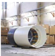
jacking pipe in front of intermediate jacking station
